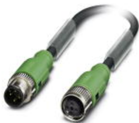
Sensor/actuator cable, 4-position, Variable cable type, shielded, Plug straight M12 SPEEDCON, A-coded, on Socket straight M12 SPEEDCON, A-coded, cable length: Free input (0.2 ... 40.0 m)
