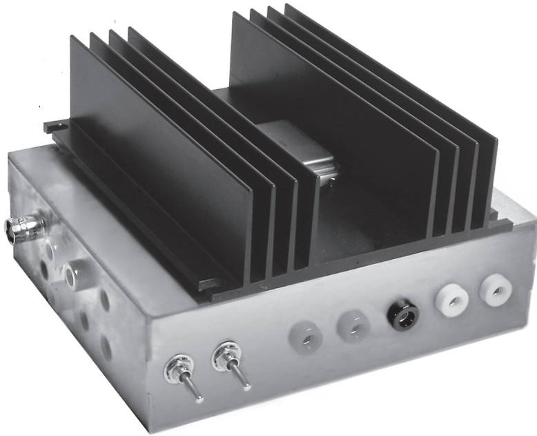
Figure 3: Inside of assembled box. Holes for components on long side were user drilled.
