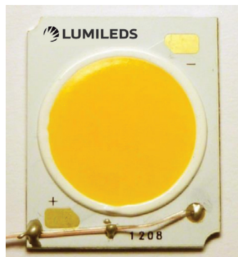
Figure 7. The recommended temperature measurement point T_s is located on the circular gold pad at lower right hand corner of LUXEON CoB emitter on the PCB.
