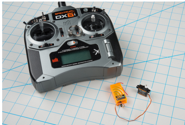
RC transmitter (top left), with receiver and steering servo.
