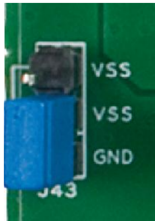
Figure 4-8. Jumper Setting for Ground Reference
