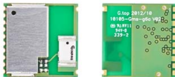
Figure 1-2: Built-in Chip Antenna Module: Carrion 2 (Gms-g6a)
