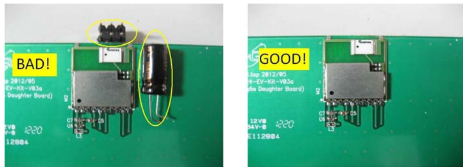
Figure 2-26: First Example of bad and good GNSS module placements
