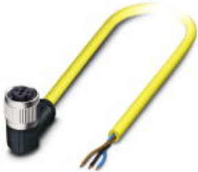
Sensor/Actuator cable, 3-position, PVC, yellow RAL 1021, free cable end, on Socket angled M12 SPEEDCON, A-coded, Cable length: 15 m
