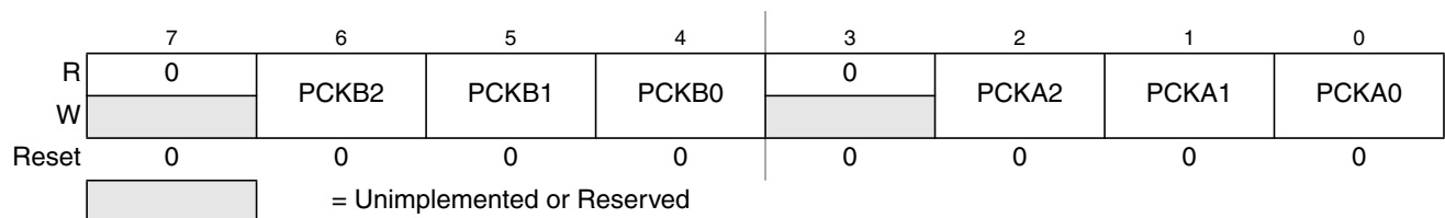
Figure 19-6. PWM Prescale Clock Select Register (PWMPRCLK)
