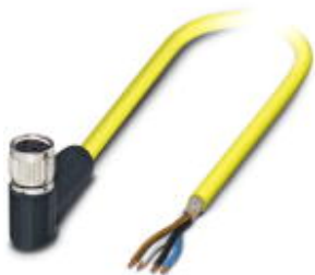
Sensor/Actuator cable, 4-position, PVC, yellow, shielded, free cable end, on Socket angled M8, Cable length: 2 m
