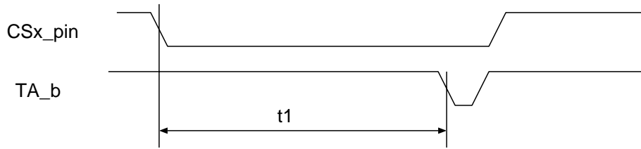
Figure 13-4 Non-IORDY Controlled IDE/SmartMedia TA Timing
