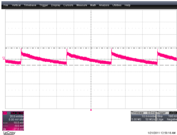
Figure 26. V_{O\_RIPPLE} = 28\text{mV} , 5V Output at 90V AC and No-Load Condition, CH2: V O (20mV/div), Time: 10ms/div
