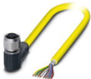
Sensor/Actuator cable, 8-position, PVC, yellow, shielded, free cable end, on Socket angled M12 SPEEDCON, A-coded, Cable length: 5 m
