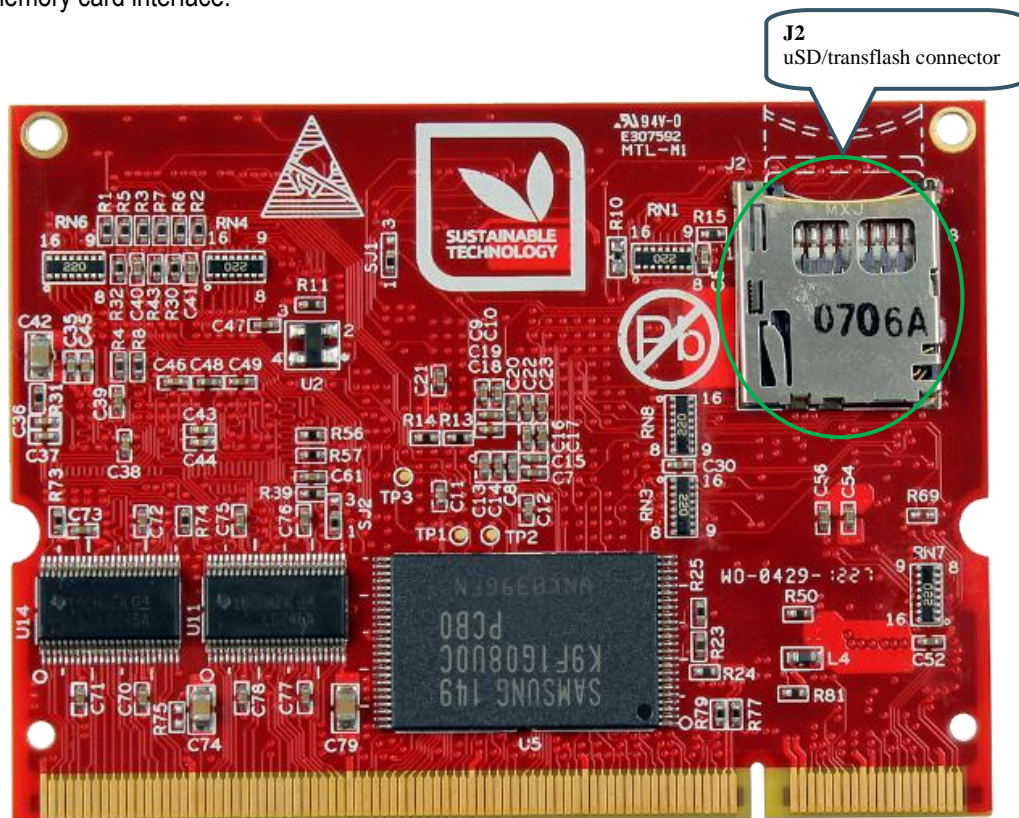
Figure 2 – LPC4357 OEM Board Picture, bottom side
