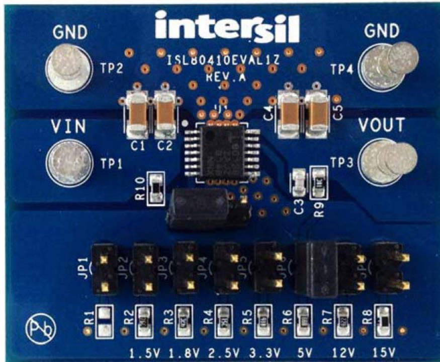
Figure 2. ISL80410EVAL1Z Evaluation Board (Top)
