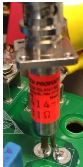
Figure 7. Low side current measurement
