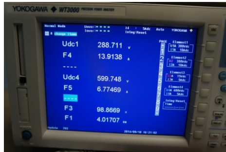
Figure 11. Efficiency data for this EVL board
