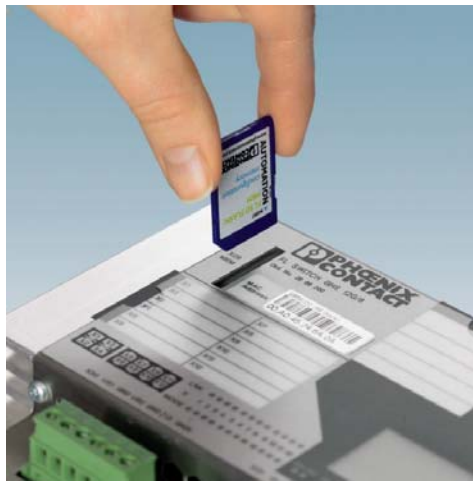
Figure 18-1 Inserting the SD card
