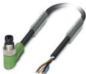
Sensor/actuator cable, 4-position, PUR halogen-free, black-gray RAL 7021, Plug angled M8, on free cable end, cable length: 1.5 m
