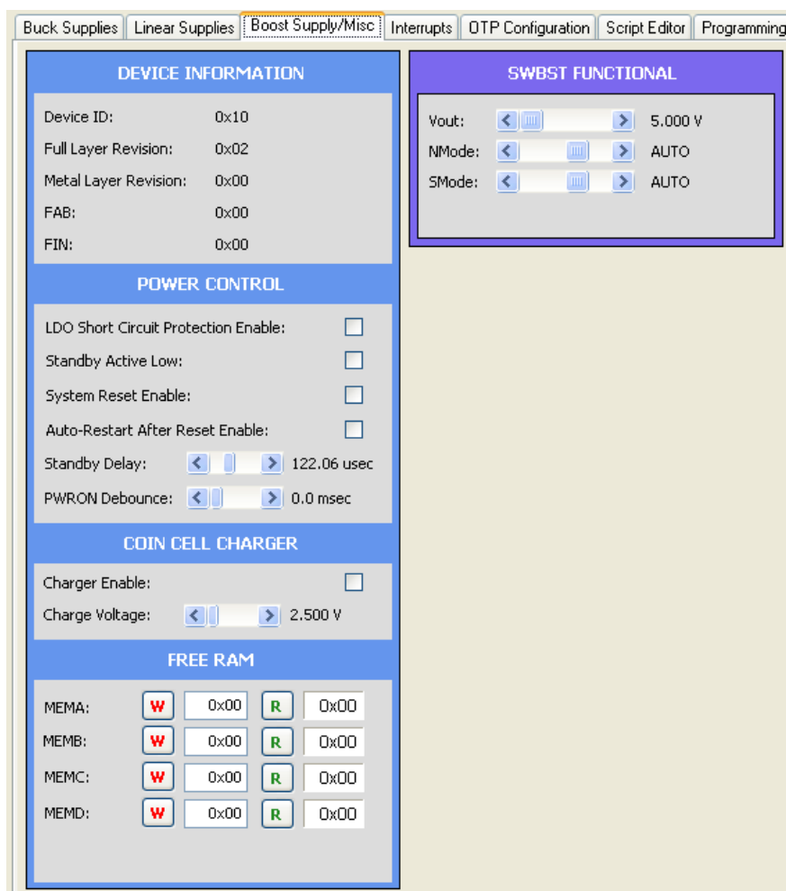
Figure 9. Boost Supply/Misc Control Tab
