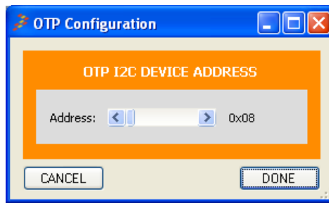
Figure 17. I 2 C Device Address
