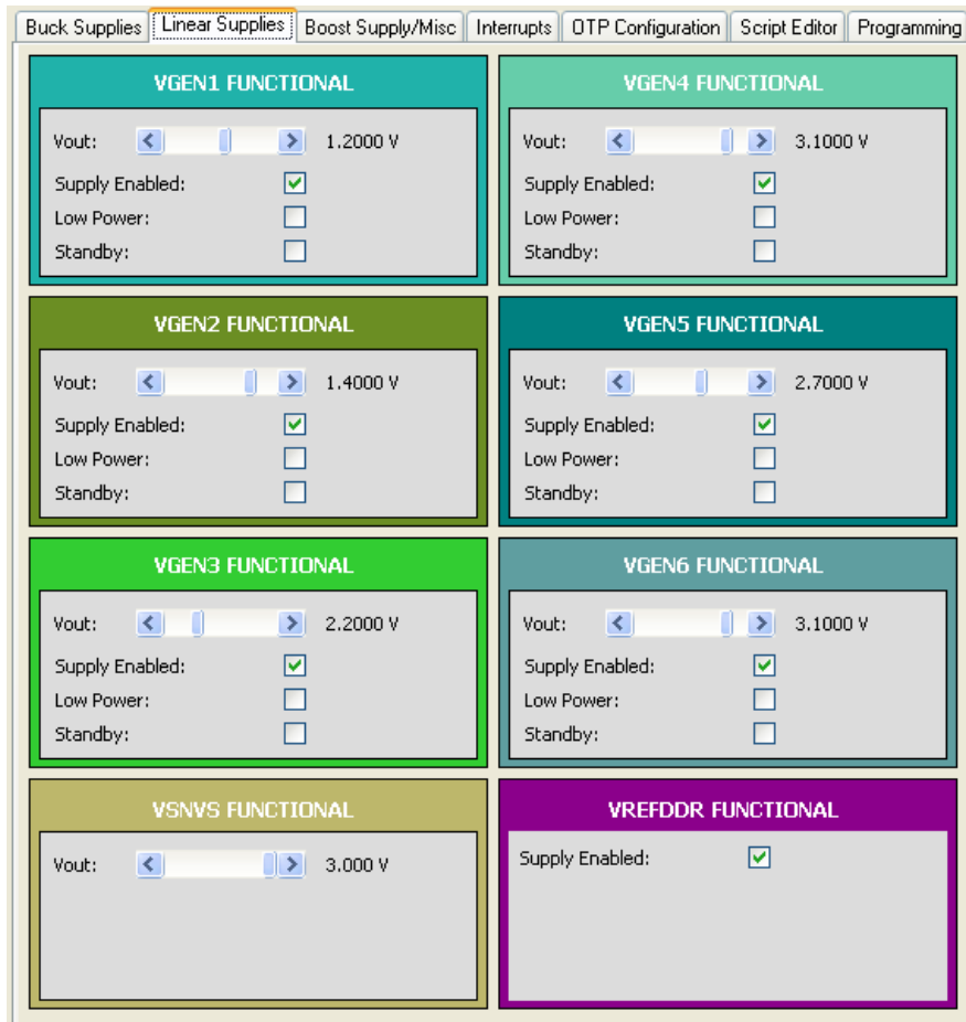
Figure 7. LDO Control Box
