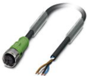
Sensor/actuator cable, 4-position, PUR halogen-free, black-gray RAL 7021, free cable end, on Socket straight M12 SPEEDCON, A-coded, cable length: 1.5 m
