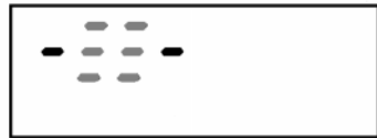
Display Indicates that the Left Reed Switch is Selected. The Gray Segments Would Be Flashing.
