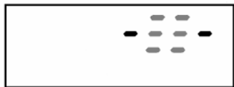
Display Indicates that the Right Reed Switch is Selected. The Gray Segments Would Be Flashing.
