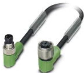
Sensor/actuator cable, 4-position, Variable cable type, Plug angled M8, on Socket angled M12 SPEEDCON, A-coded, cable length: Free input (0.2 ... 40.0 m)
